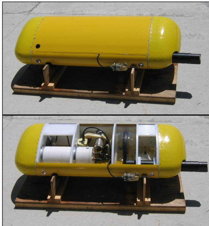
Fig. 2. The Aqualog carrier. The lower photo shows the carrier without the cowl.
