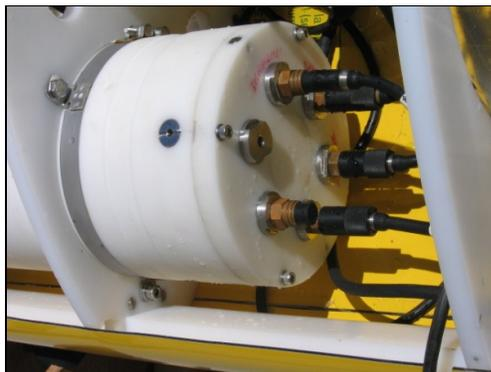
Fig. 3 The housing for the carrier electronics including the battery pack.
